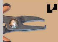
Specially designed tool for front cutting, suitable for access in dense areas of PCBs. It cuts the component lead at 1.5mm from the surface.
